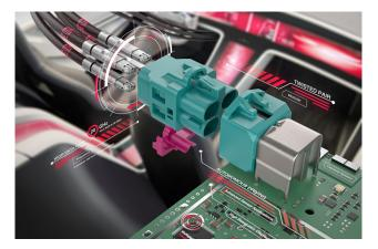
An example from an innovative portfolio: Rosenberger's highspeed data connector systems, used in driver assistance systems and autonomous driving applications, are applied in components such as cameras and displays. (Source: Rosenberger)
